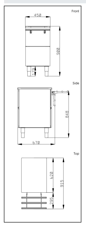
Flexy Compact Ambient Unit on cupboard (1 GN) with one stainless steel tray slider
